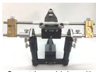
Connect the condyle bars with adjustment adhesive again by using the adjustment tool and the Reference Calibration key
